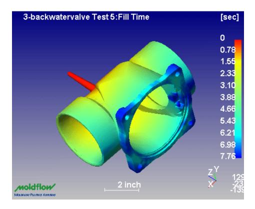
Confidence of Fill: The results of this analysis help determine whether the part will fill with a high level of confidence and also indicate the areas of low confidence of fill. The analysis simulates the molding parameters at the normal processing range for the material selected from the database.
